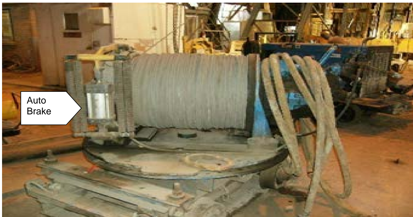
Figure 8: Portable Air Tugger with Auto brake
