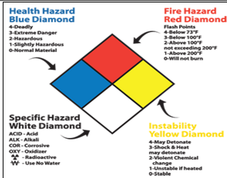
Figure 3: Hazard Ratings (NFPA 704)
