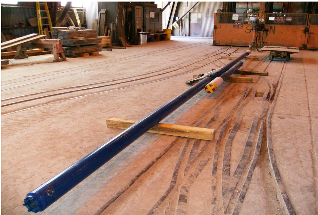
#1. MOTOR AND SEAL READY TO BE LOWERED AT YATES SHAFT
