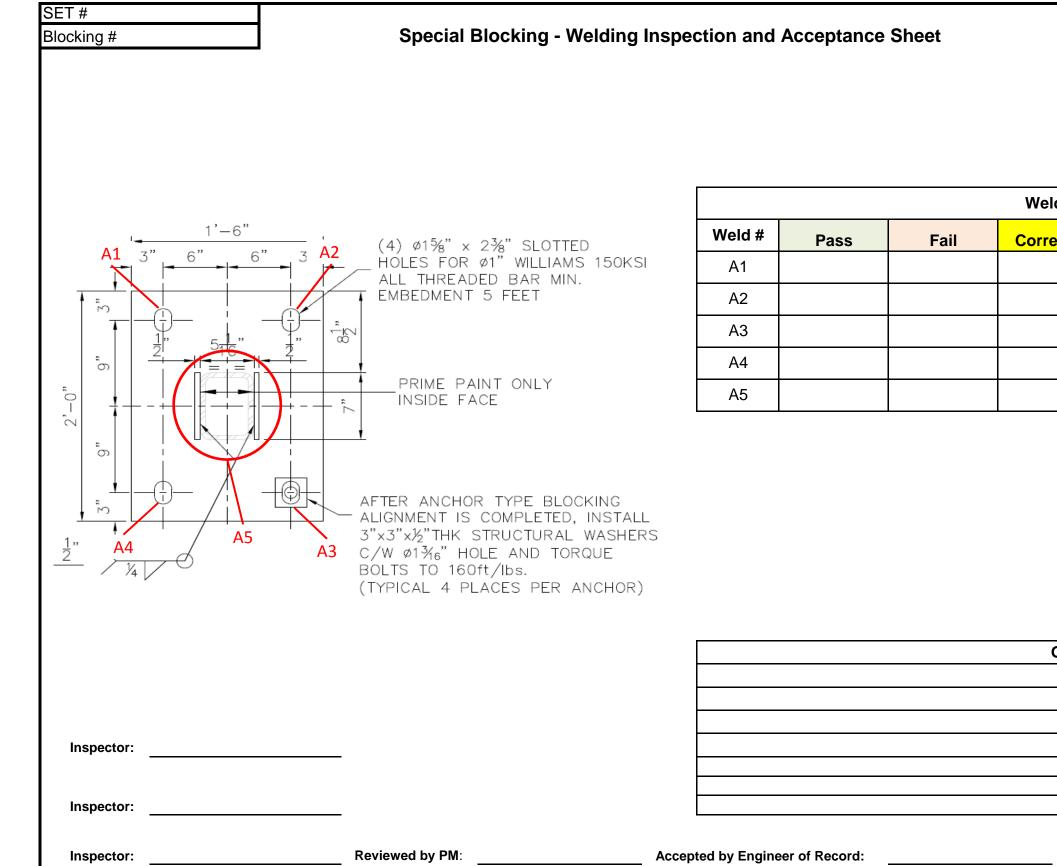
Weld Inspection Check Fail Corrected Pass Corrected
