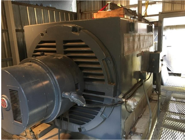
Figure 5 G.E. 3,000 HP Synchronous Motor
