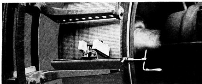
FIG. 21—GRINDING DEVICE FOR TRUING COMMUTATORS
